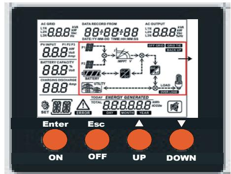
All AC and DC currents: input and output per phase, load in %,
